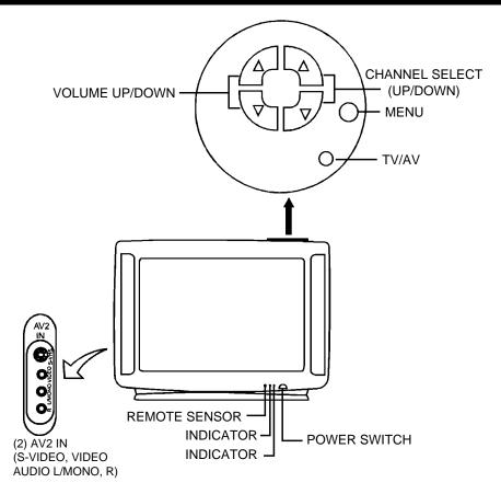
Note:\* Functions of MENU, TV/AV, VOL ▲/▼, CH ▲/▼, are also provided to the remote controller.
